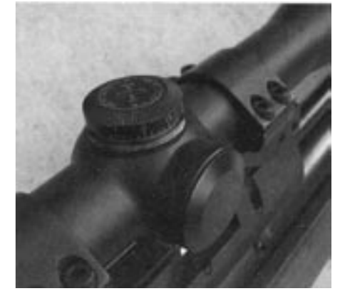
Left: Lynx's new 1.5-4.5x24 (top). Like the 1-3x20 (centre), its eye-relief measures 120mm at maximum magnification. The mounted 3-10x40 is shown for comparison. Centre: The 4.5-14x Lynx can be set parallax-free at 15m - ideal for air rifle use. Right: The dials are finger adjustable for easy operation and sport the so-called 'zero-storing' facility.
