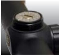
Remove the cap by rotating anti-clockwise, and use a screw-driver or coin to rotate the control to adjust for windage and elevation. The graduated range scale may be turned to indicate zero position.
