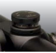
Remove the cap by rotating anti-clockwise, and rotate the control to adjust for windage and elevation. Loosening the locking thumb-screw atop the knob and pulling the knob upward disengages the adjustment mechanism and enables you to reseat the knob in the zero position. Once the control is zeroed hand-tighten the locking thumb-screw back into place. A rotation indicator scale is engraved on the shaft beneath the control knob.
